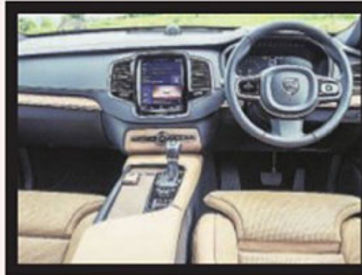
Most controls have been moved to the centre display; rear seating area is very spacious; headlights have been inspired by Thor's hammer; controls are done in a diamond-knurled finish
