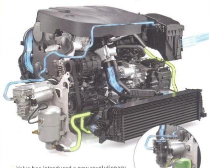
Volvo has introduced a new revolutionary technology with its new D5 diesel engine called the PowerPulse. A powerful and electrically driven air compressor and a pressurised air tank
