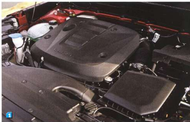
1. The 2.0-litre Volvo diesel engine makes its way into the XC40 as well but in its D4 trim - producing max power of 190bhp and peak torque of 400NM. 2. Wireless charging in keeping with the times 3. Harman Kardon music system with 13 speakers
