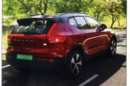
With a 0-100 time of just 4.9s, a XC40 Recharge treads on sportscar territory. But it is not a surprise given the max torque of 660Nm available from standstill. Pedal to
